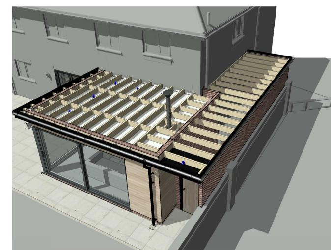
2425 Corner post clad in insulated boards to match doorset
